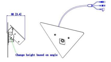
1. Loosen the bolt and separate it from the plate. Loosen the nut and separate camera module and base bracket.
